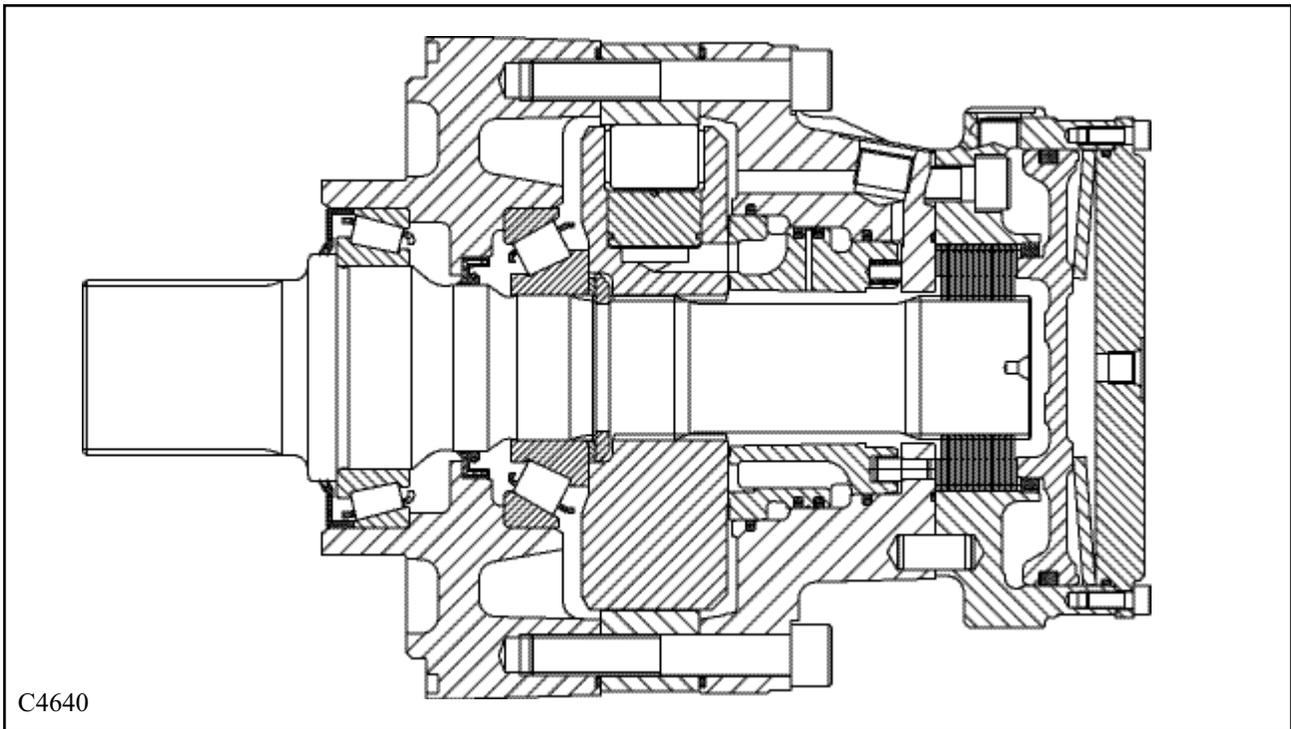
The basic radial piston design uses a combination of mechanical and hydraulic principles that are utilized in the high torque, low speed motors.
