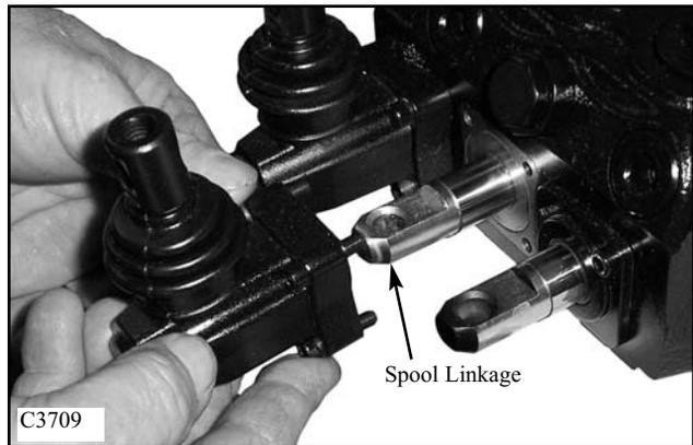
5 Pull out the spool. (fig. C3713) As you pull out the spool, note it's smooth action as it comes out of the valve body. The spool should move freely and smoothly in the bore of the valve body. Check the control valve spool and bore for scuff marks or abnormal wear. Replace the spool and or control valve if signs of wear are present.
