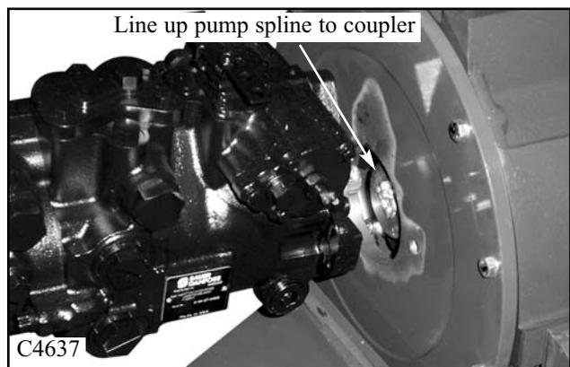
Line up pump spline to coupler
