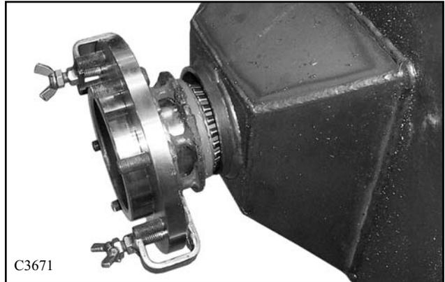
12 Place the rear (inside) axle bearing onto the axle. (fig. C3813 & fig. C3814)
