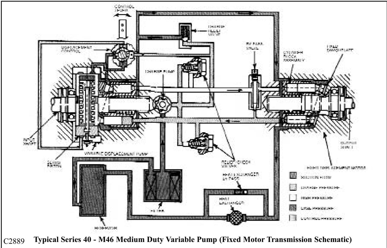
C2889 Typical Series 40 - M46 Medium Duty Variable Pump (Fixed Motor Transmission Schematic)
