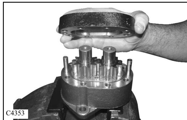
6. Remove the idler shaft and drive shaft from its bearing bore. Inspect the journals and the flat faces top and bottom of the gears. Ensure these surfaces are free from burrs or scratches. If scratches are found, clean them with a flat stone and/or a very fine emery cloth. Rewash the gears with light oil after this operation.
