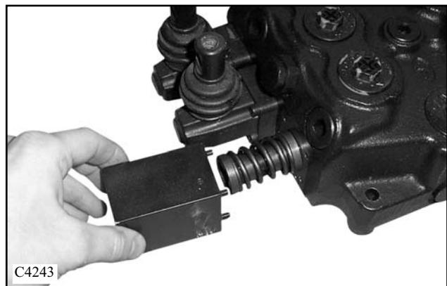
6 Remove the solenoid spool assembly from the control valve. (fig. C4244) Note the effort required to remove the spool from the spool bore. It should come out smoothly without binding or “snagging” throughout it’s travel.
