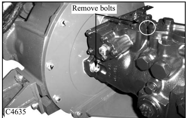
12. Use the mechanical lifting device to take the weight off the tandem. Slide the tandem pump splined shaft out of the adapter coupling on the engine. Remove the pump from the loader.
