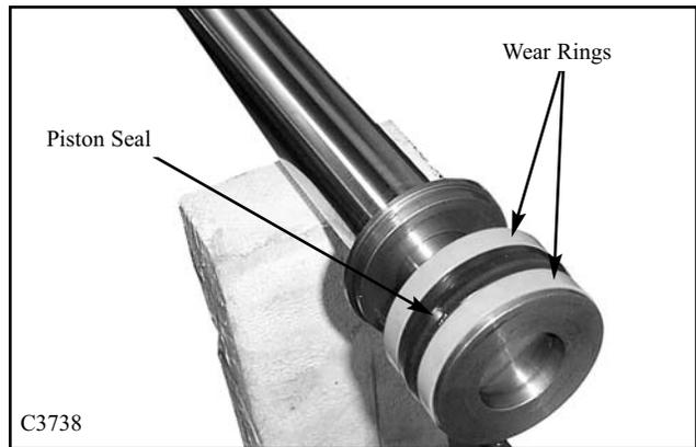
7 Install the piston assembly to the cylinder rod. Some rear piston assemblies are threaded onto the cylinder rod. Use a spanner wrench to install the rear piston part to the cylinder rod. Torque the lock nut to the rod at 250-275 ft lbs (339-373 Nm). (fig. C3740)
