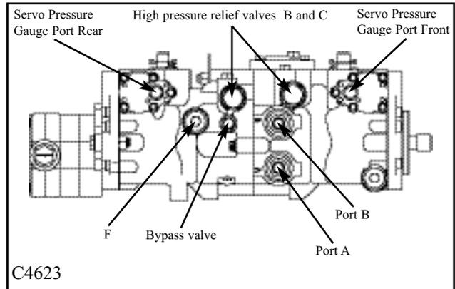
**NOTE:** Internal charge pump model shown
