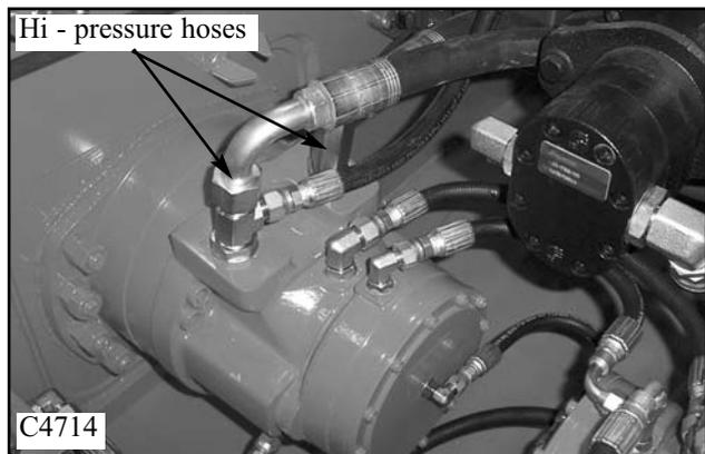
10 Install the adapter fitting to the brake lines and case drain. Connect the hoses to the brake line, case drain and 2 speed (if applicable) on the torque motor.(fig. C4645) Torque the fittings and hoses according to the torque chart in section 2.13 page 2-33.
