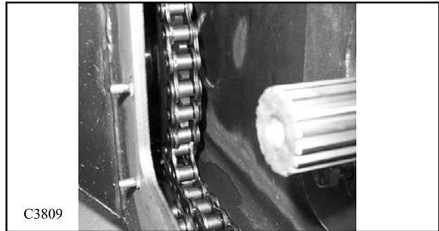
3 Place the ends together and install the new connecting link so that the cotter pins face away from the inspection cover. (fig. C3810). Bend the ends of the cotter pins at least 90 degrees.
