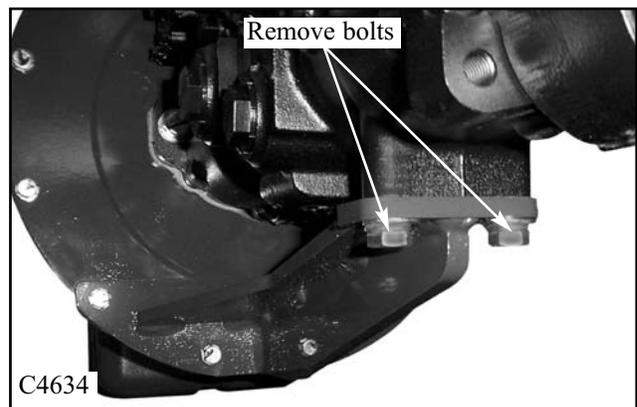
10. Remove the 2 bolts from the rear pump mount located on the front of the engine. (fig. C4635) Inspect the bolts and the matching threads in the pump mount assembly for damage, repair or replace if required.
