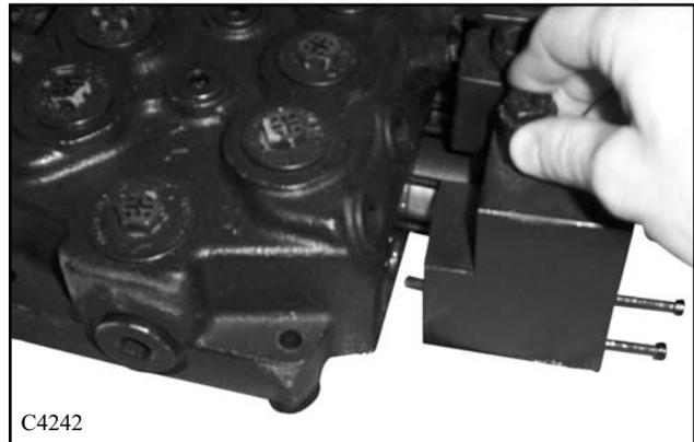
5 Remove the screws and the bottom end cap from auxiliary section.(fig.4243) Upon assembly torque the screws to 5 ft lbs (7 Nm)
