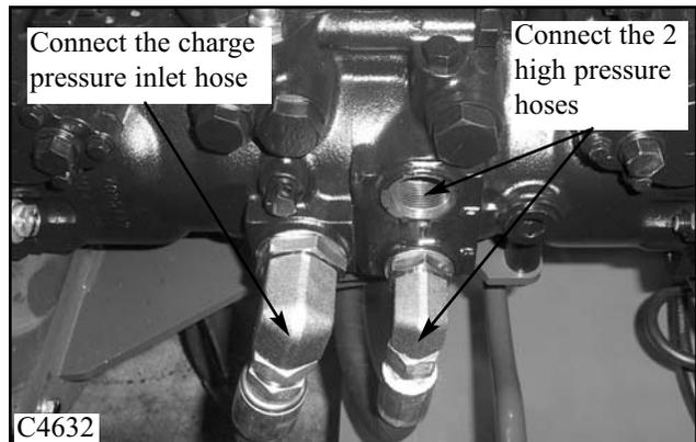
Connect the charge pressure inlet hose
