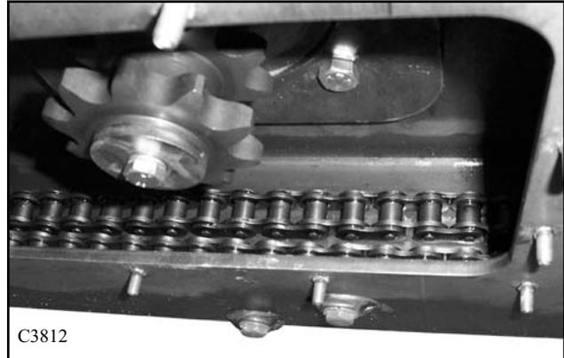
2 Place one end of the front chain over the top of the front axle sprocket. Rotate the axle and bring the chain along the bottom of the final drive housing to approximately the center. (fig. C3809) Wrap the other end of the chain around the motor sprocket teeth closest to the motor.
