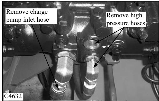
8. Remove the hose from the case drain and the 2 high pressure hoses for the RH torque. (fig. C4633) Mark the hoses if necessary to ease re-assembly. Remove the fitting from the pump and keep in a clean area. Inspect the fittings and o-ring for damage, replace as required. Cap all open ports and lines.
