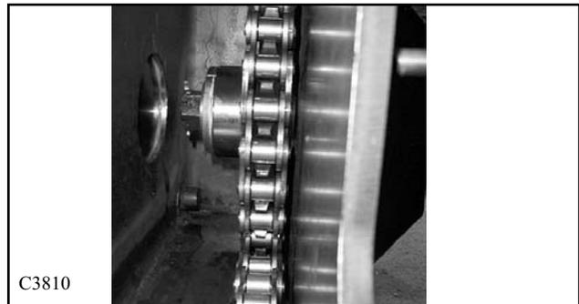
4 Wrap the rear chain over the rear axle sprocket. Rotate the axle and chain around the bottom of the final drive housing and around the bottom of the motor sprocket closest to the inspection cover opening until the ends of the chain meet together.
