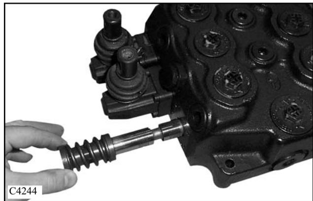
7 Inspect the spool and spool bore for abnormal wear. (fig. C4245) Replace the spool and / or the control valve if large scratches or indentations are present in the spool or spool bore. Minor scratches can be removed from the spool with extra fine emery cloth.
