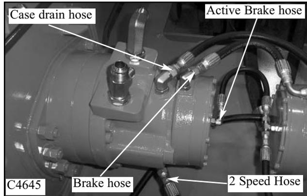
9 Install the high pressure adapter fittings to the drive motor ports.
